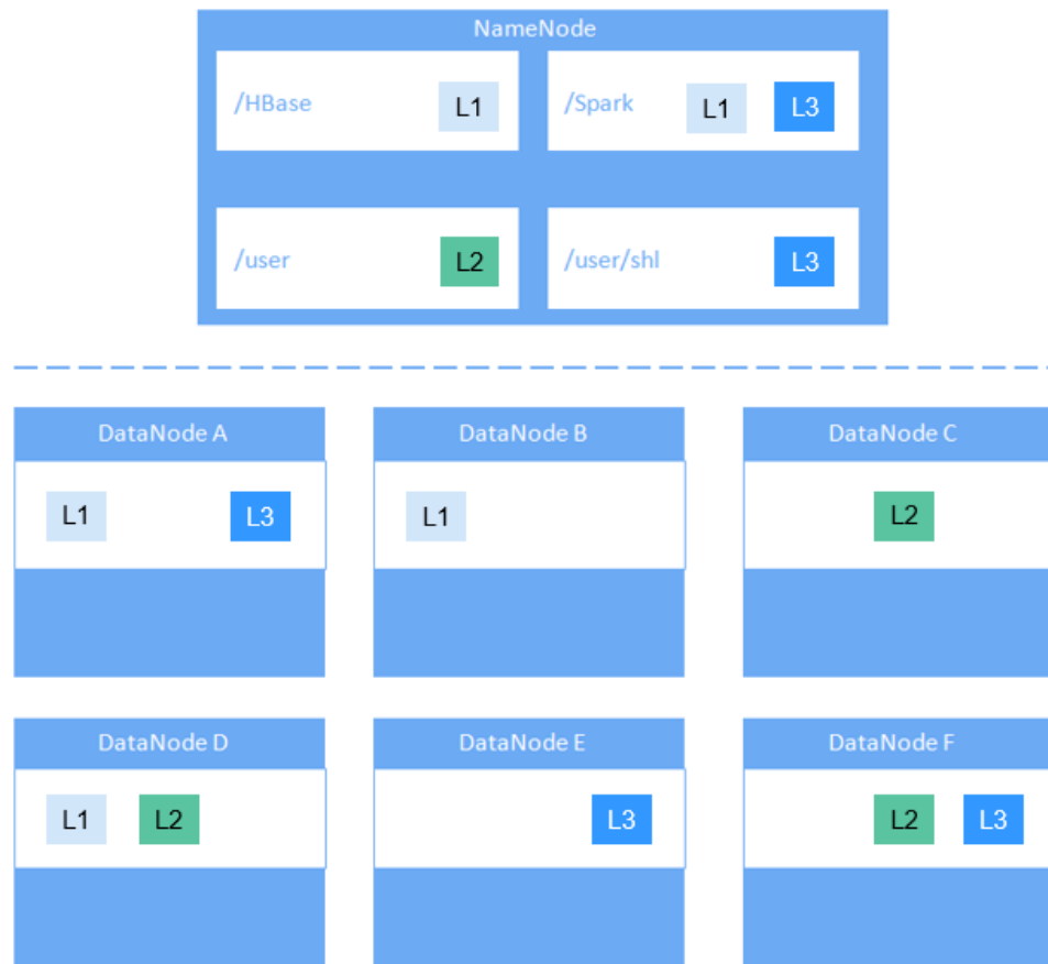
Figure 1-58 Example of label-based block placement policy
